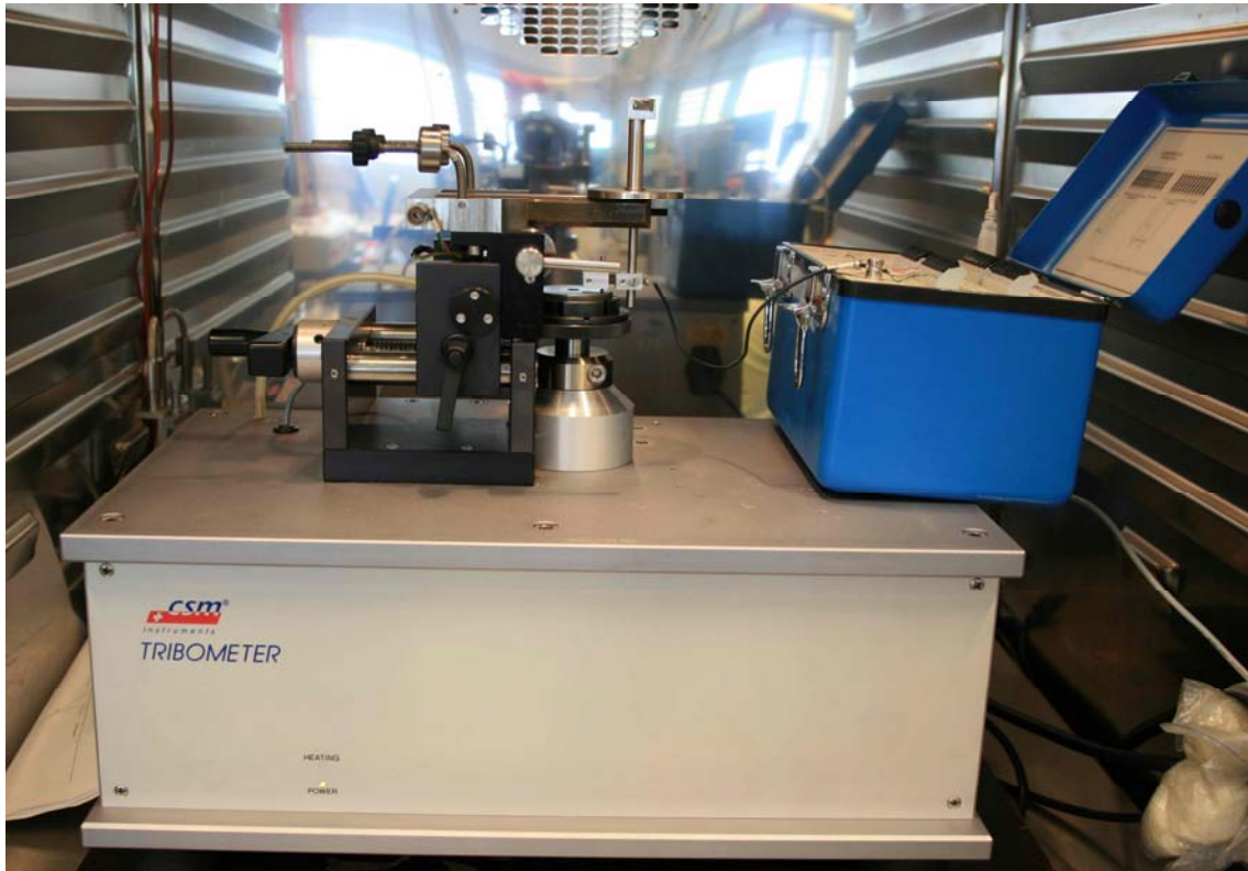
Figure 4. The final ensemble made of: CSM tribometer, new pin on disc microtribometer and Vishay strain recorder
