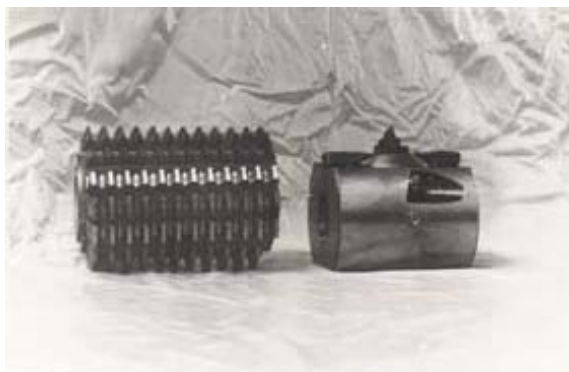
Figure 8. Single tooth gear hob
