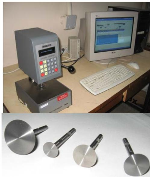
Figure 2. Geometry of Brookfield viscometer
